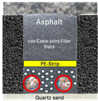
Covering the empty cable duct with PE cord/PE strips/quartz sand prevents damage if the cable sheathing is removed during a later repair.
