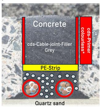
\*for optimal adhesion of the sealing compound on the concrete, please prime the concrete edges before grouting
